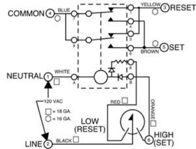
Contact Ratings: SPDT dry relay contacts, 10 A, 125 VAC.
